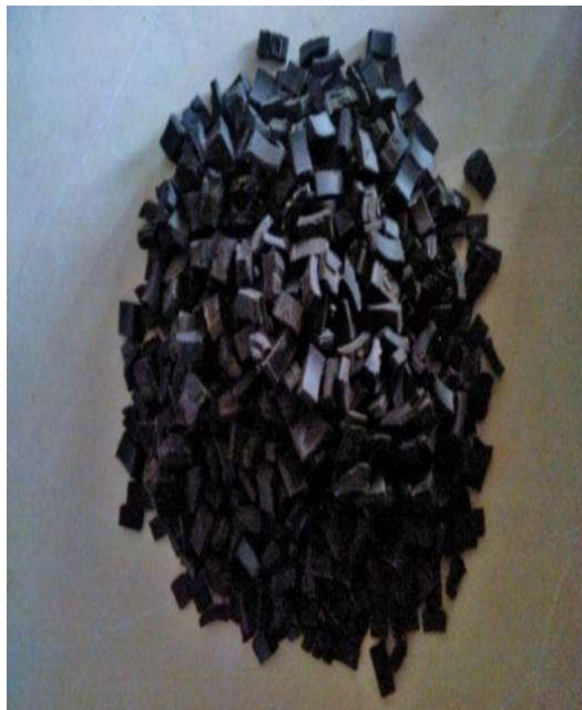
3.1 WASTE TYRE RUBBER AGGREGATE
